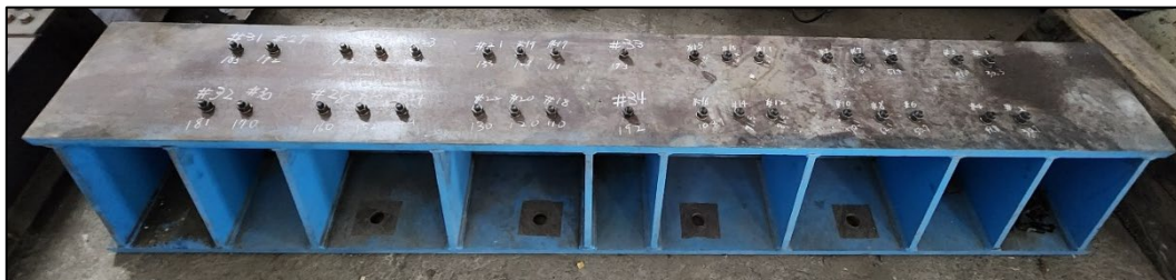
Fig. 7 Footing beam tap-tone test
